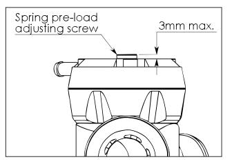
Making the springs softer will allow the valves to open easier and vent longer, and increasing the preload means you will need to drive the car harder (i.e. more boost) before you start to hear the BOVs venting, and the blow-off sound will be shorter in duration.
