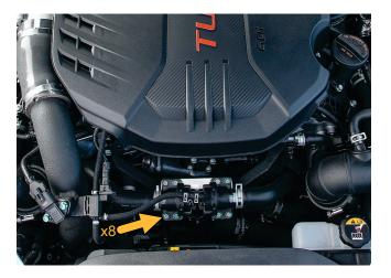
2) Ensure the brown o-rings are installed in the grooves on the underside of the Hybrid valves, then install both valves onto the engine using the supplied screws and 5mm hex key. The valves are oriented so the vacuum nipples point to the front of the car as shown below (please note, Respons valves shown, but vacuum orientation is the same for the Hybrid valves).
